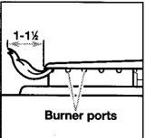
size and shape as shown. A good flame is blue in color not yellow. If the flames are not burning at all ports, you may need to clean the burner ports.
